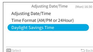
Step2. Press "^" or "v" to select the setting and press "OK".
