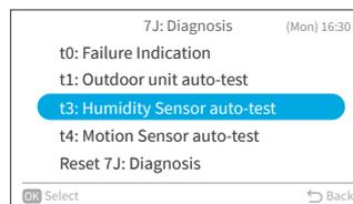
Step2. Select "Yes" and press "OK" to request humidity sensor auto-test. Then it returns to Step1.
