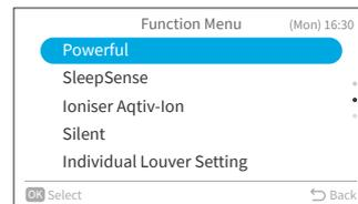
Step2. Select "Yes" and press "OK" to start powerful operation. Powerful operation ends in 20 minutes. Then the system automatically operates with the previous settings used before powerful operation.
