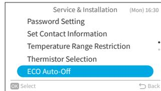
Step2. Press "v" to select "Auto-Off Timing" and press "OK".
