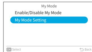
Step2. Press "^" or "v" to select desired mode and press "OK".
