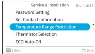
Step2. Select "Upper/Lower Limit for Cooling Operation"/"Upper/Lower Limit for Heating Operation"/"Upper/Lower Limit for Auto mode" and press "OK".
