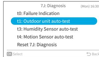
Step2. Select "Yes" and press "OK" to request outdoor unit auto-test. Then it returns to Step1.
