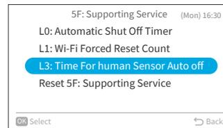
Step2. Press "^" or "v" to change the human absence detection time, then press ">" to select "OK" and press "OK". Then it returns to Step1. Adjustment value of absence time until Auto off execution is as follow.
