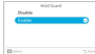
Step3. After mold guard is enabled, you will see an icon "Mold Guard" displayed on the home screen.
