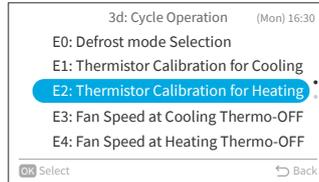
Step2. Press "^" or "v" to change the thermistor calibration for heating, then press ">" to select "OK" and press "OK". Then it returns to Step1.
