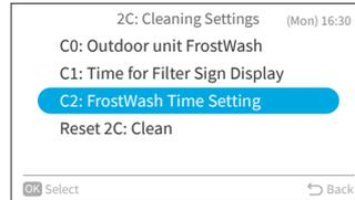
Step2. Press "^" or "v" to change the indoor unit auto FrostWash startup time, then press ">" to select "OK" and press "OK". Then it returns to Step1. Adjustment value of cumulative air conditioner time until execution of indoor unit auto FrostWash is as follow.
