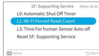
Step2. Press "^" or "v" to change the reset count, then press ">" to select "OK" and press "OK". Then it returns to Step1.
