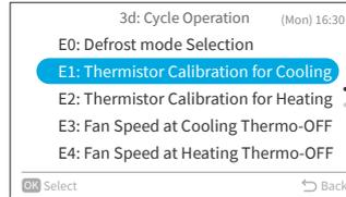
Step2. Press "^" or "v" to change the thermistor calibration for cooling, then press ">" to select "OK" and press "OK". Then it returns to Step1.
