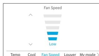
Step2. By pressing "^" or "v", the fan speed changes as follows.
