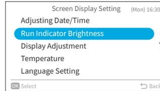
Step2. Press "^" or "v" to change the brightness value. Select "OK" and press "OK", the screen returns to the "Screen Display Setting" screen.
