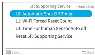
Step2. Press "^" or "v" to change the timer value, then press ">" to select "OK" and press "OK". Then it returns to Step1.
