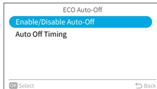
Step3. Press "^" or "v" to select "Disable"/"Enable" and press "OK" to enable/disable Auto-Off.
