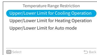
Step3. Press "<" ">" to select the setting limit, then press "^" "v" to change the temperature value.
