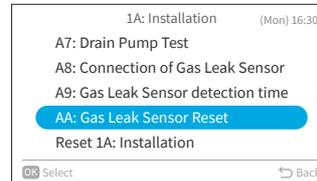
Step2. Select "Yes" and press "OK" to reset gas leak sensor.
