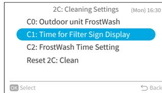
Step2. Press "^" or "v" to change the cumulative amount of time the air conditioner takes to display the filter cleaning recommendation sign, then press ">" to select "OK" and press "OK". Then it returns to Step1. The cumulative time of adjustment value is as follow:
