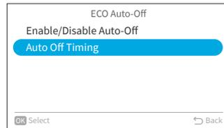
Step3. Press "^" or "v" to change the time from 20min to 120min, then press ">" to select "OK" and press "OK".
