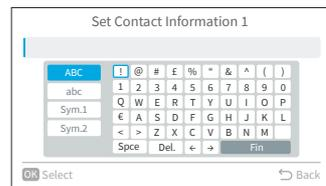
Step3. Press ">" to move cursor to the keypad. Press "^", "v", "<", or ">" to select the font and press "OK" to register it. (Up to 60 characters can be used for each contact information.)
