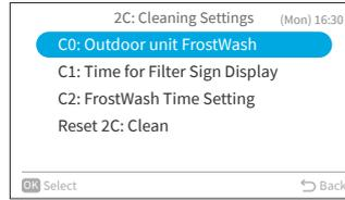
Step2. Select "Yes" and press "OK" to launch Frostwash cleaning of outdoor unit. Then it returns to Step1.
