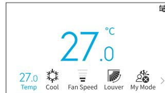
Step2. By pressing " $\wedge$ ", the temperature is increased in increments of 0.5°C(1°F) to a maximum of 32°C(90°F).
