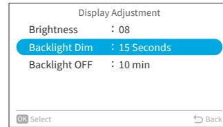
Step3. Press "^" or "v" to select the dim time intervals and press "OK". The item changes as follows:
