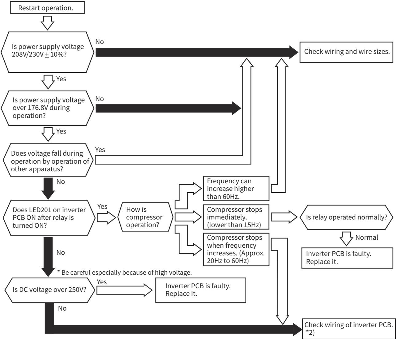
\*1): If there is high residual voltage, make sure to perform high voltage discharge according to the item 1.2.4 (2) "Checking Method for Rectifier Circuit".
