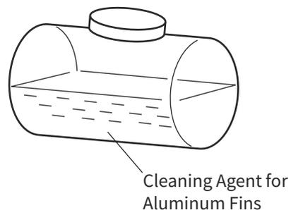
(8) Insert the spray nozzle through the hole of the cleaning water collector. Operate the water pump and clean the dust on the heat exchanger. After cleaning, spray clean water to remove the cleaning water. Adjust the pressure of the water pump so as not to damage the fins.
