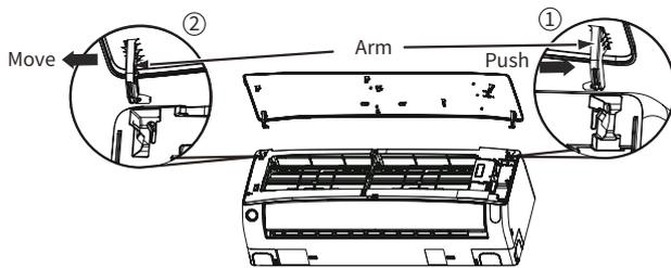
1. Push the end of the right-side arm outward to release the tab.
