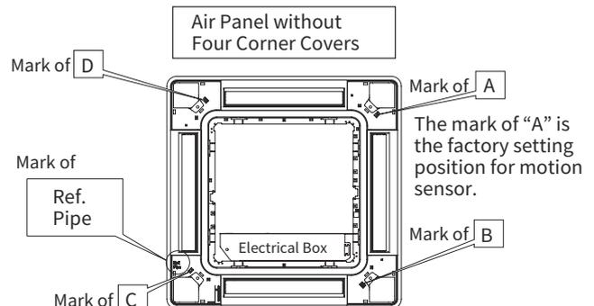
The motion sensor cannot install to the location of the mark of "C" .
