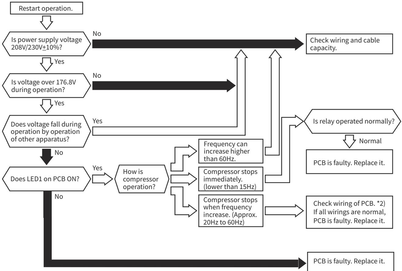
\*1): If there is high residual voltage, make sure to perform high voltage discharge according to the item 1.2.4 (2) "Checking Method for Rectifier Circuit".
