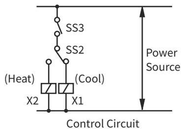
**Wiring Diagram Example of Fixing Operation Mode**
