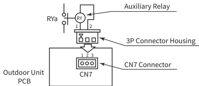
**Wiring Diagram Example of Operation Signal**
