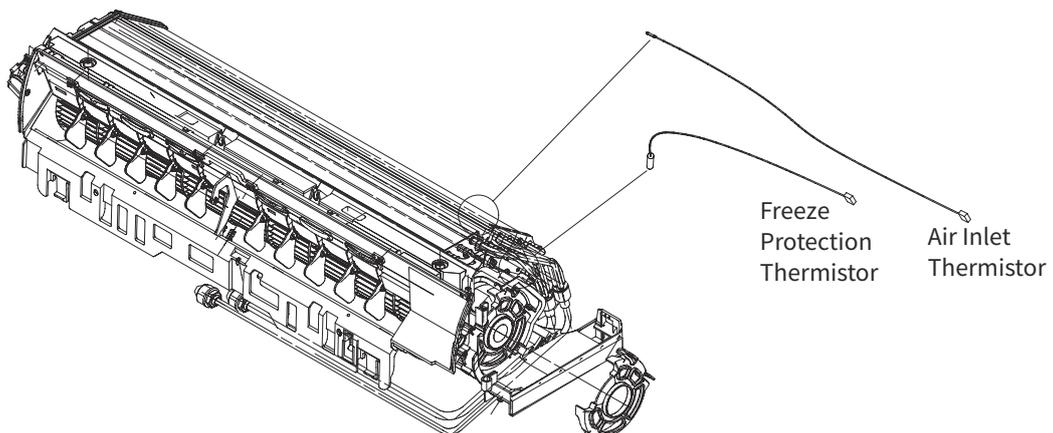
(2) Thermistor for Indoor Suction Air Temperature (For Room Temperature Control)
