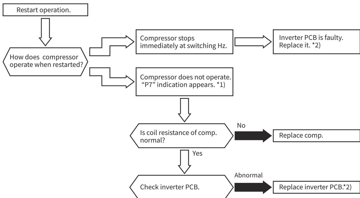
\*1) The indication appears on 7-segment display of the outdoor unit PCB.
