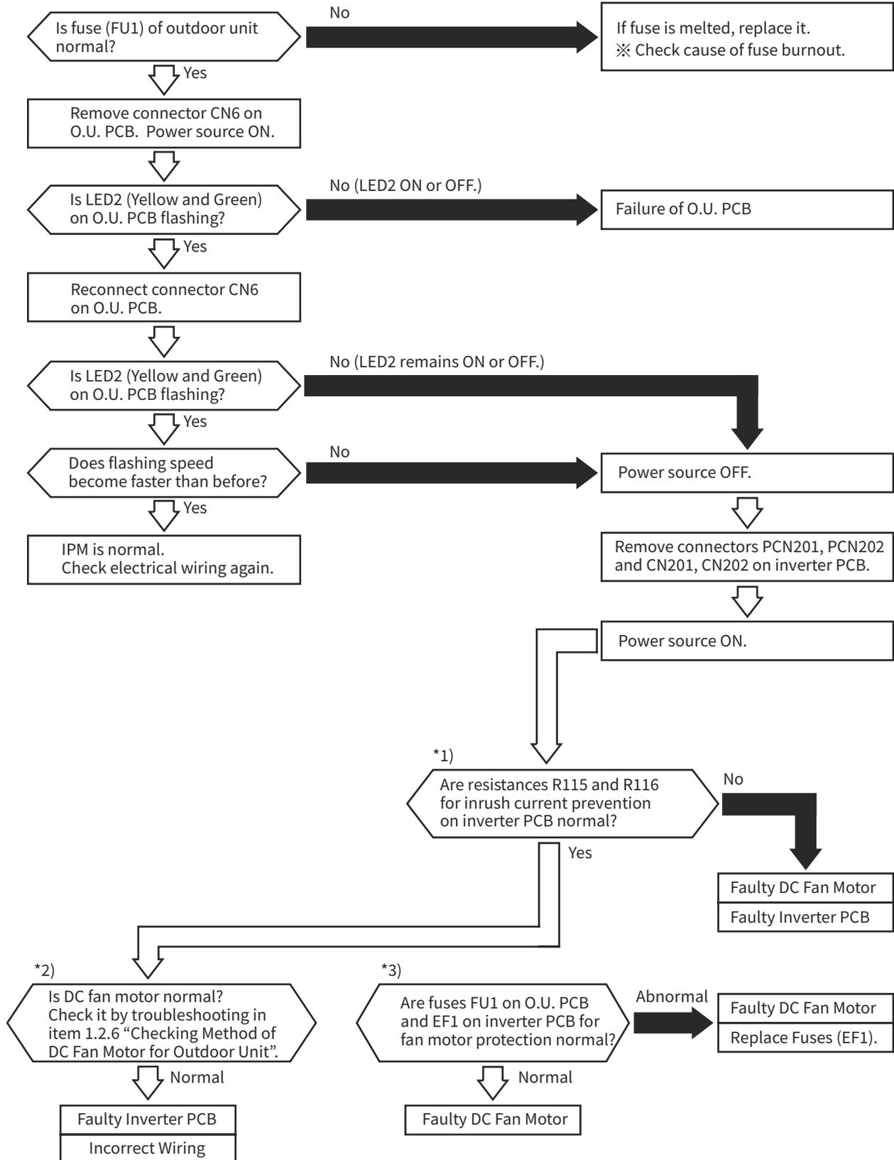
\*1): Surely perform the troubleshooting of the resistance for inrush current prevention (R115/R116) on inverter PCB. If the resistance for inrush current prevention (R115/R116) fails, the transmission failure occurs.
