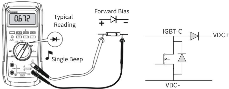
Remove all the terminals of the inverter PCBA before check.
