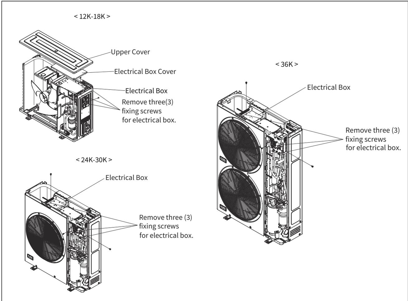
Remove the electrical box after disconnecting wires.
