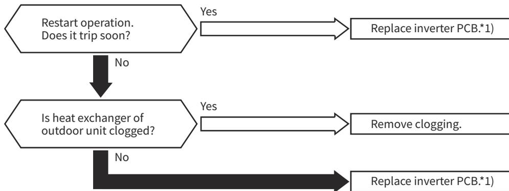
\*1) The maintenance and replacement for inverter PCB should be performed after performing surely the voltage discharge work according to the item 1.2.4 (2) "Checking Method for Rectifier Circuit".
