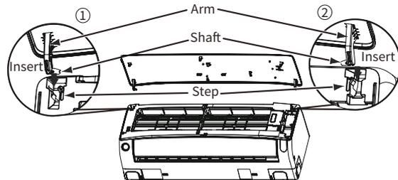
1. Insert the shaft of the left arm along the step on the unit into the hole.
